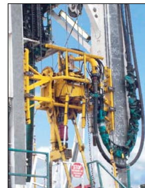
Foremost Explorer III-50 equipped with F-100T top drive
