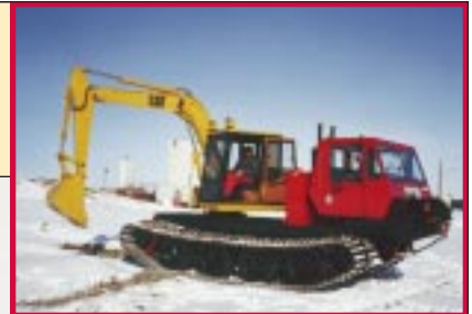
Nodwell 240 with backhoe for pipeline maintenance
